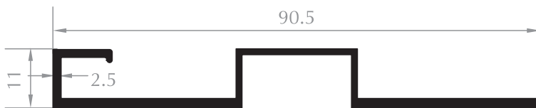
CEPHE PROFİLİ FACADE PROFILE Kod/Code :CE4001 Ağırlık/Weight:0,536 kg/m
