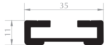
MOBİLYA PROFİLİ FURNITURE PROFILE Kod/Code :MB1038 Ağırlık/Weight:0,470 kg/m
