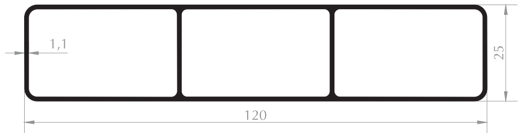
MOBİLYA PROFİLİ FURNITURE PROFILE Kod/Code : MB1043 Ağırlık/Weight : 0,985 kg/m
