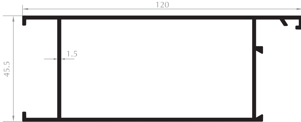
BAZA ETEK PROFİL KICK PLATE PROFILE Kod/Code : DO2010 Ağırlık/Weight: 1,336 kg/m
