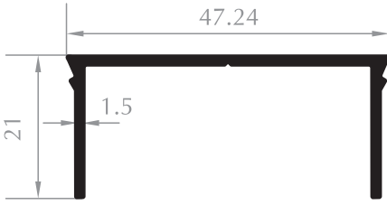
BASKI PROFİLİ COVER PROFILE Kod/Code :CE4028 Ağırlık/Weight:0,367 kg/m
