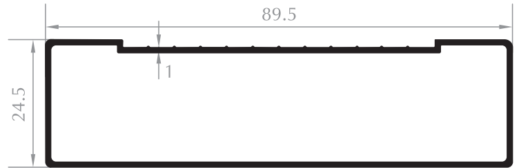
MERDİVEN PROFİLİ STAIRS PROFILE Kod/Code :MH1926 Ağırlık/Weight:0,611 kg/m
