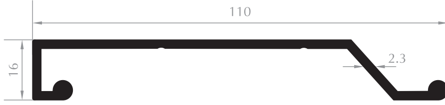
ASKI PROFİLİ HANGER PROFILE Kod/Code :CE1101 Ağırlık/Weight:0,921 kg/m
